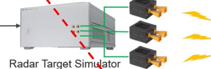
Radar Sensor (DUT)
